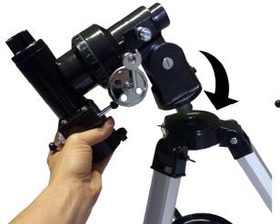
Rotate the declination axis of the mounting upwards, if needed, and attach the telescope tube ring.
