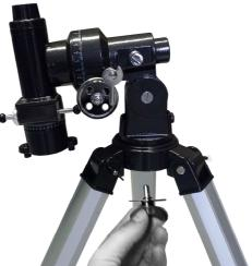
To do that, unscrew both screws from the mounting socket for the telescope tube ring.
