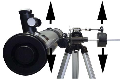
Depending on if the tube or the counterweight sinks down, move the counterweight on the rod to achieve a balance. If you achieved that, then secure the counterweight and close the right ascension clamp.
