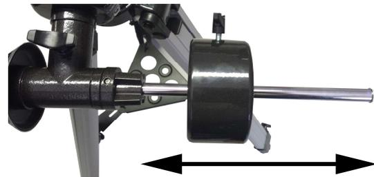
You've now adjusted the right ascension axis. That means that this axis will now always be level, independent from the position the telescope is in.
