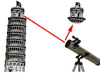
Look through the viewfinder tube. If you do not see exactly the same image, adjust the viewfinder tube. On the search tube you will find small screws, which can be used to adjust the viewfinder tube until the object can be seen exactly in the viewfinder tube. Then you have aligned telescope and finder telescope parallel to each other. If you encounter the viewfinder, repeat the procedure. The viewfinder should be set up before each observation.
