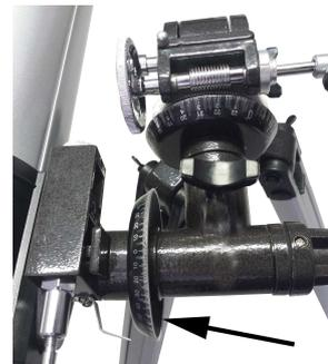
To correct that, slightly open the clasp of the telescope tube ring, so that the tube can be moved back and forth. Move the tube until it doesn't move anymore by itself (meaning it won't slump down on one side) and then close the declination clamp again.
