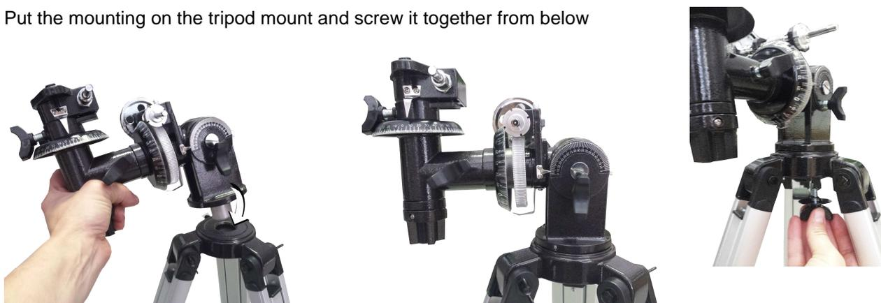
Rotate the declination axis of the mounting upwards, if needed, and attach the telescope tube ring. To do that, unscrew both screws from the mounting socket for the telescope tube ring.
