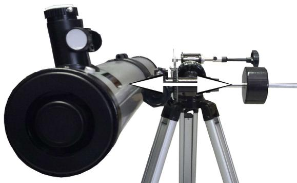
Loosen the right ascension clamp. It holds the axis. If you loosen this clamp, then the axis is freestanding and can be moved like a seesaw.
