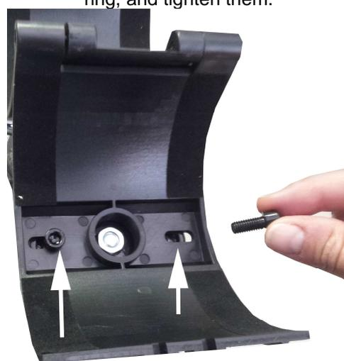
Attach the fine movements shafts.
