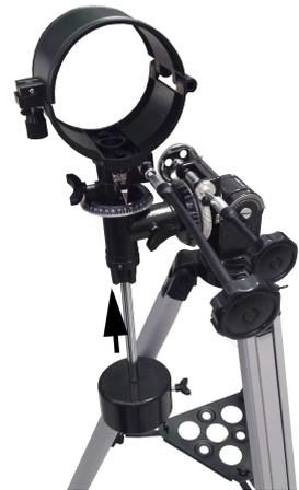
Put the tube into the telescope tube ring and close the telescope tube ring at the side. Make sure that the declination shaft is pointing towards the ocular.
