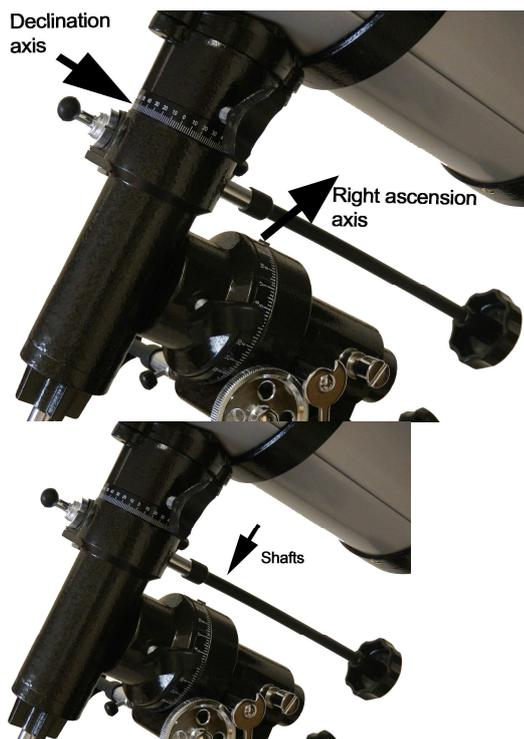
The adjustment of the mounting is important, because both axes have to stand level. This has the effect that the telescope, no matter how it's positioned, won't tip over sideways due to the unilateral overload. Think of a seesaw: if one side has more load on it, then it will sink downwards.
