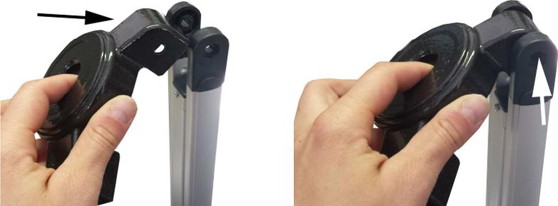
Also especially ensure when setting up the tripod leg that the mounting for the ocular shell is on the inside!
