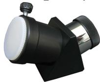
The picture is upside down and inverted in astronomical telescopes. The star diagonal is righting the picture again, so that you can also comfortably make nature observations, but it doesn’t correct the inverted image. It deflects the optical path by 90 degrees, so that it’s easier to observe objects near the zenith through the ocular.
